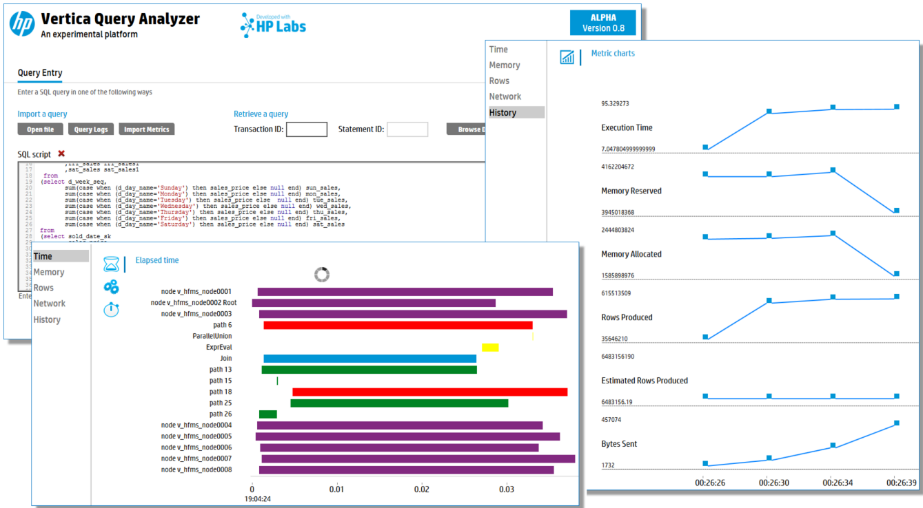
Figure 2: VQA entry (top left), chart view (bottom left), and history (right) for an execution of the TPC-DS Query-2
