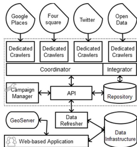
Figure 2. CitySense architecture
